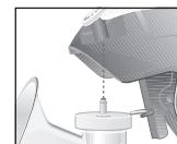
7. Take the pump unit **2** and push the intake fitting of the lid **4** **completely** into the suction connector on the pump unit **2** (fig. ⑨).
